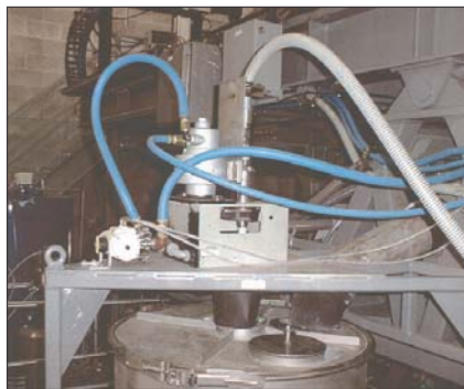
Inside a macerator, high-pressure waterjets break down warhead material.
