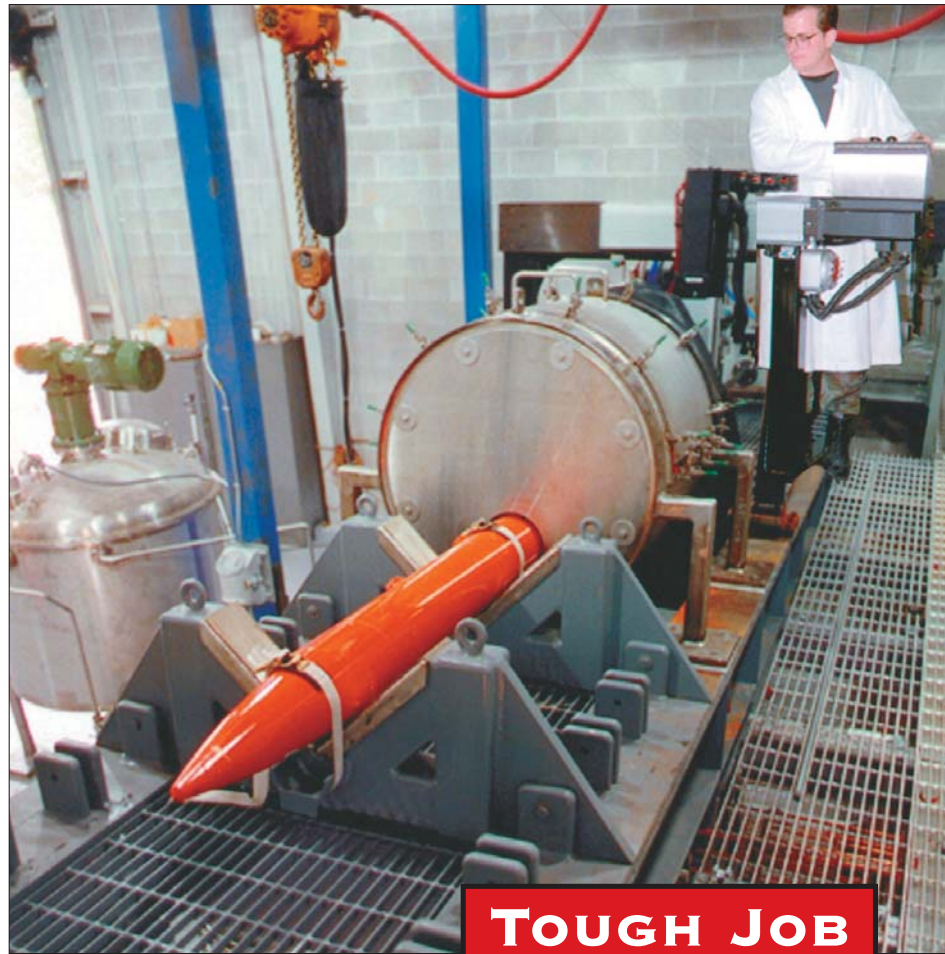
A research technician at Eglin Air Force Base prepares to demilitarize a warhead through hydro-mining with high-pressure waterblasting equipment supplied by Aqua-Dyne Inc.
